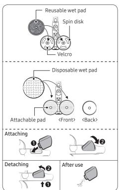
Use to clean a wood and linoleum floor with a wet pad.
