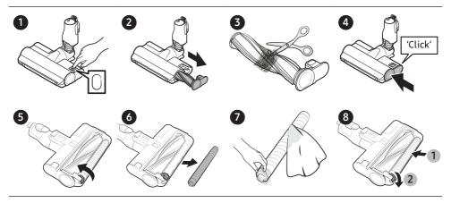
If the foreign matter is not removed, use scissors to remove it.
